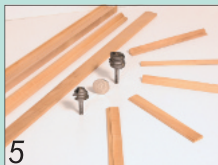
5 Miniature multi-profile cutters can create a huge range of profiles. Note the 50p piece for scale
