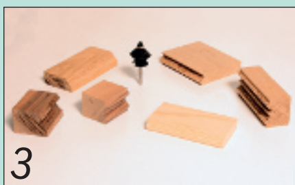
3 All these profiles in boards of different thicknesses were made with the T2940 cutter
