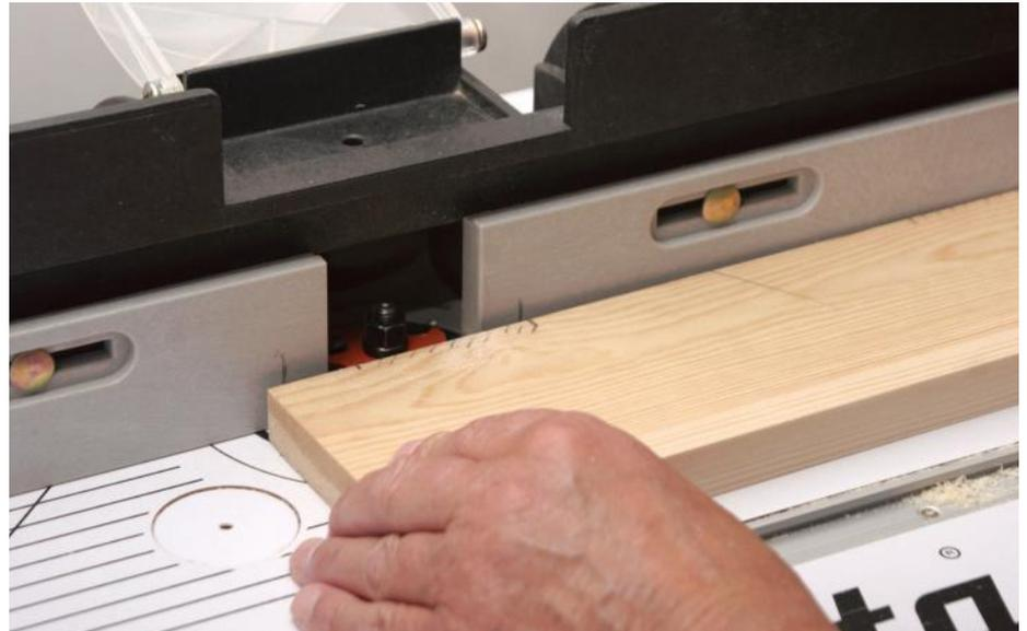
**7** Pivoting the board into the cutter. Note pencil marks on fence. The guard is raised here for photographic clarity
